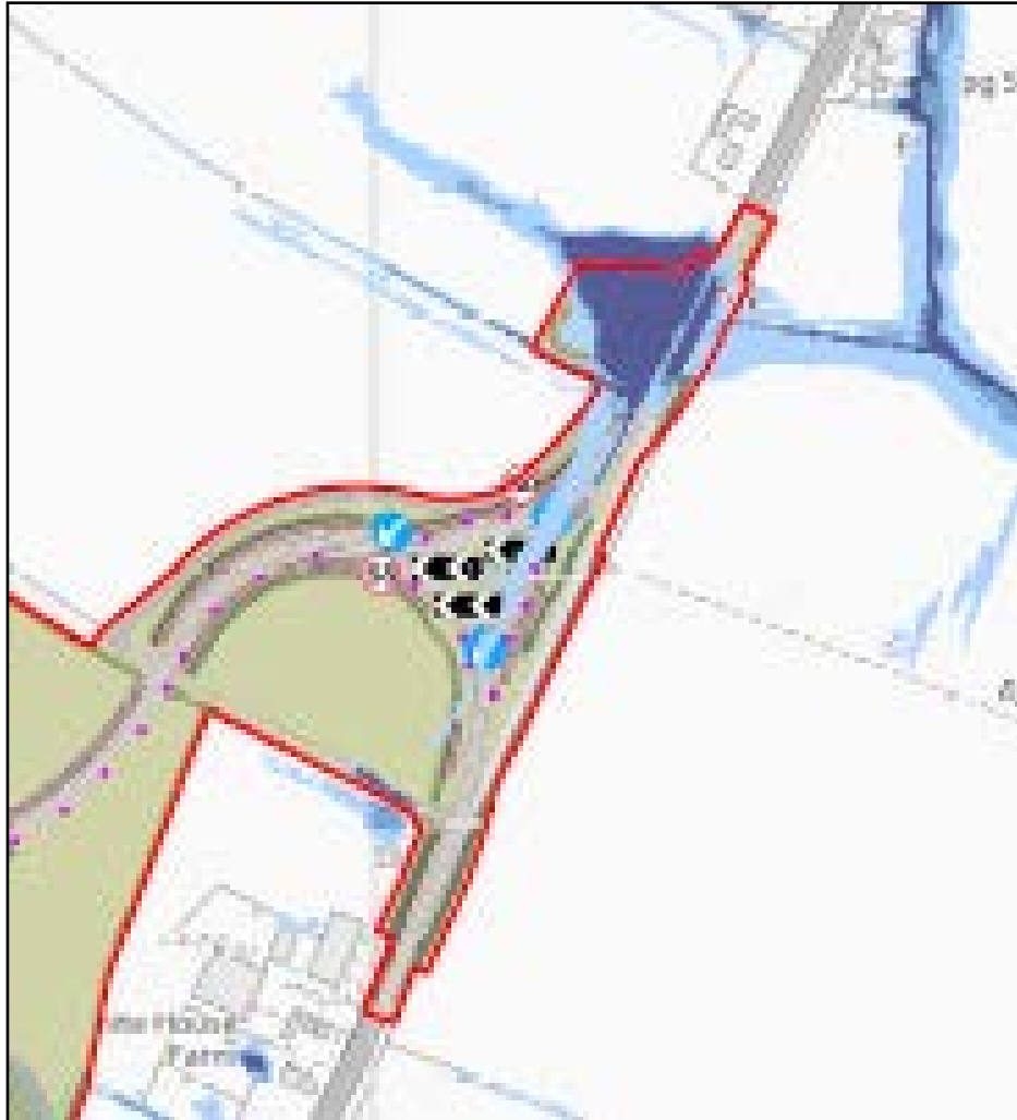
Plate 6: A12 predicted surface water flood risk locations at roundabout northern tie in
