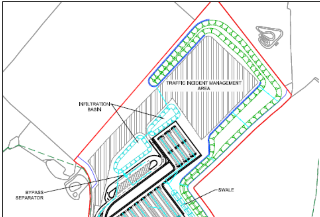
Plate 1: Southern park and ride internal layout showing concept drainage infrastructure to the north
